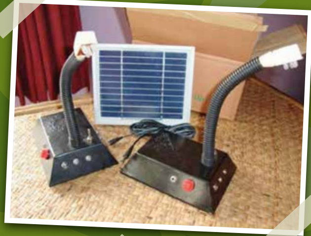
LED lamp with a battery and small solar panel
